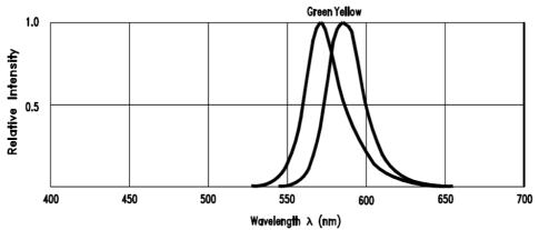
Fig.1 Relative Intensity vs. Wavelength
